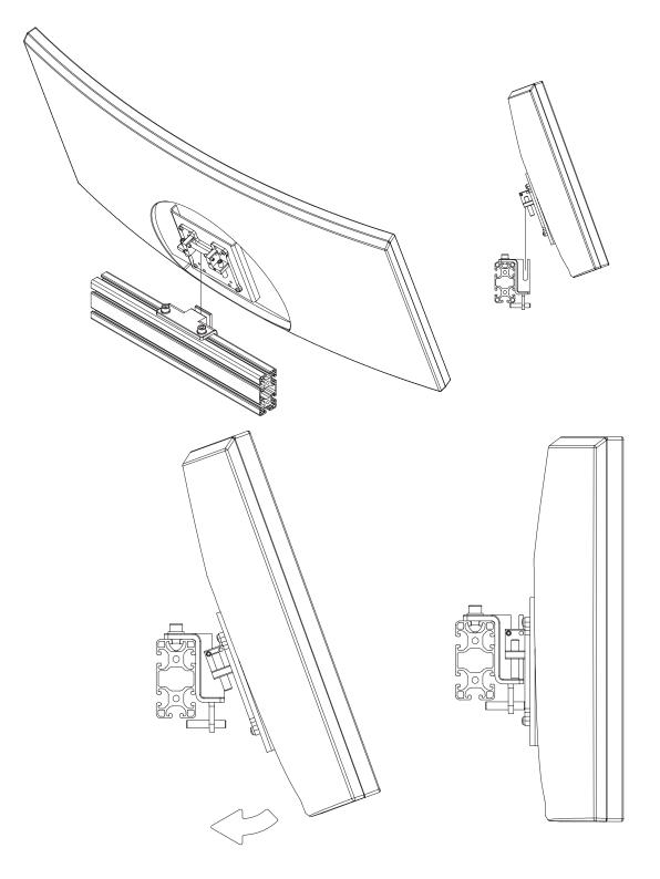
Drop the pin (A4) into the slot and carefully angle the monitor downwards to rest on the end of part A12.
